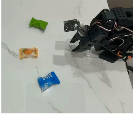
Figure 8: The hardware setup: an SO-101 arm with commodity servos over a flat work surface, with three candies as the referent set. Raw phone footage; no fixture, no calibrated lighting, no motion capture.
